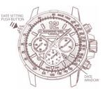
In order to adjust the date rapidly, press the date setting buton until the required date appears in the window at 4:30.
