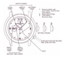
Your RAYMOND WEIL watch may be fitted with a screw-down crown. Before setting the time or changing the date, it is therefore necessary to unscrew the crown by pulling it straight out and turning it anti-clockwise. The crown will then be released by a spring. After completing all settings, press lightly on the crown, while turning it clockwise, and screw it back in gently in order to preserve your watch's water-resistance.
